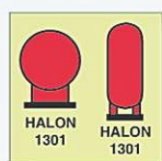
Halon 1301 bottles in protected area PV 6050 JJ
